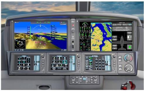
In the cockpit, three touchscreen avionics controllers power two large main display screens.
